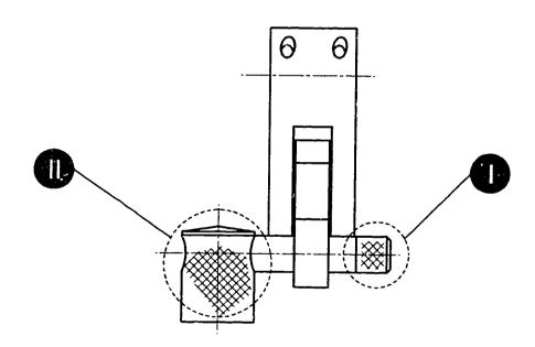
Driving pin and sliding piece Visual inspection, area II
